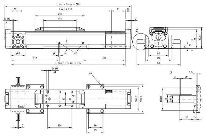
A1: depth 9, Heli coil A2: lubrication holes
