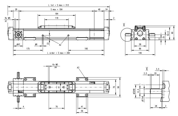
A1: depth 10, Heli coil A2: lubrication holes
