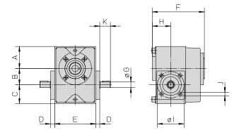
The worm gear is installed directly to the unit and require no intermediate coupling between the two. To be able to install the gear to the motor a bell house flange must be used between the gear and the motor. The bell house flange, which includes a matching coupling, is ordered separately. A shaft cover can be ordered to cover the second primary shaft on the gear in case it is not being used.
