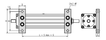
The mounting feet option can be mounted on the unit from the factory if this is stated in the ordering key at order (ECT series only) or be ordered seperately using the part number (T and ECT series). When ordered seperately all neccessary screws to attach the feet are included. Note! The distance "G" can be different depending of the screw diameter of the unit.
