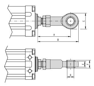
The spherical joint option can be mounted on the unit from the factory if this is stated in the ordering key at order (ECT series only) or be ordered seperately using the part number(s) (T and ECT series). When ordered seperately all neccessary componnets to attach the spherical joints to the unit are included.Type M joints includes a grease nipple. Note! when ordering a spherical joint seperately, make sure that the extension tube end has an outside thread adapter to be able to mount it.
