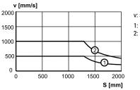
v: speed S: stroke length 1: ECT13-B63R • 3PB-4010
