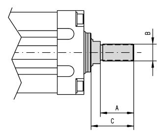
The outside thread option comes mounted from factory if this is stated in the ordering key at order. Which types that are possible for the different unit sizes depends on on the ball screw diameter of the unit, see "Ball screw diameter" in the table.
