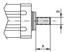
The outside thread option comes mounted from factory if this is stated in the ordering key at order. Which types that are possible for the different unit sizes depends on on the ball screw diameter of the unit, see "Ball screw diameter" in the table.
