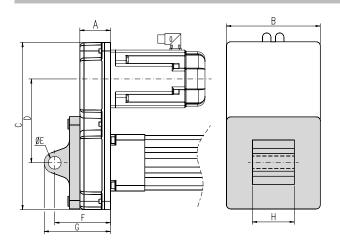
The clevis option is only available for ECT units with BGM belt gear and is orderder by stating this in the ordering key at order. The clevis comes mounted on the unit from the factory.
