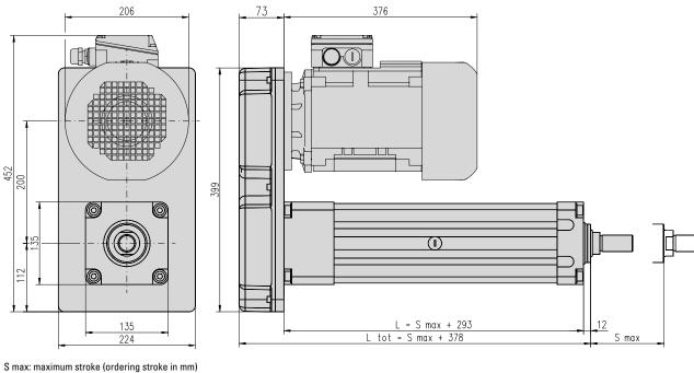
S max: maximum stroke (ordering stroke in mm) L: cover tube length L tot: retracted length
