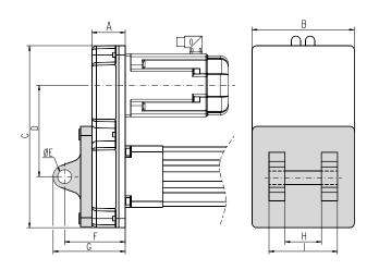
The clevis option can either be mounted on the belt gear from the factory if this is stated in the ordering key at order (ECT series only) or be ordered seperately using the part number (T and ECT series). The clevis mounting option can only be mounted on T130 or ECT130 units equipped with a BGM belt gear.
