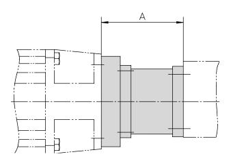
The bell house flange includes a matching coupling. Note! Keep in mind that heavy motors will need extra support in order not to break the flange or gear due to the load torque created.
