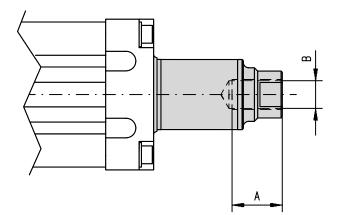
The inside thread option comes mounted from factory if this is stated in the ordering key at order. Which types that are possible for the different unit sizes depends on on the ball screw diameter of the unit, see "Ball screw diameter" in the table.
