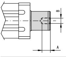
The inside thread option comes mounted from factory if this is stated in the ordering key at order. Which types that are possible for the different unit sizes depends on on the ball screw diameter of the unit, see "Ball screw diameter" in the table.
