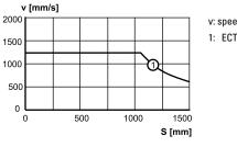
v: speed S: stroke length 1: ECT09-B53R •• LP-3220
