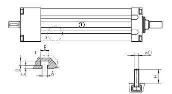
The T60, T90, T130, ECT90 and ECT130 models all have T-slots running along the entire profile. T60 has two T-slot (one on each side) while the other models have four (two on each side). Suitable T-slot bolts can be ordered using the part numbers in the table below.
