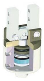
(2) Roller Guide Type: The tapered roller guide is moved by the roller to open and close the jaw. The method is applied usually to small Grippers and the product quality depends on the production precision.
