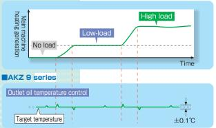
Note) Pattern diagram with the heating load stabilized at 0 - 100% (Comparison with Daikin unit)
