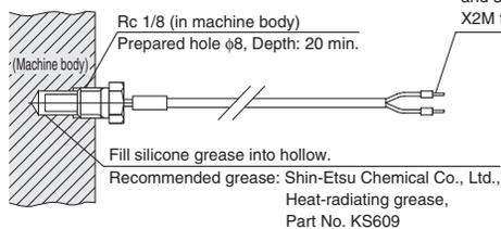
Connection to terminals 30 and 31 of Oil Cooling Unit X2M terminal block
