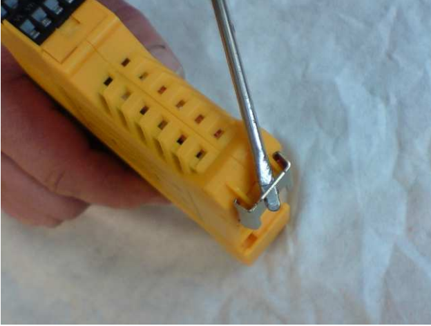
Picture 3a, 3b. For the installation on the rail pull the snapper
