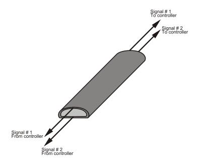
These signals are fed back to the controller via the 1x4 wire or 2x2 wire connection cable.
