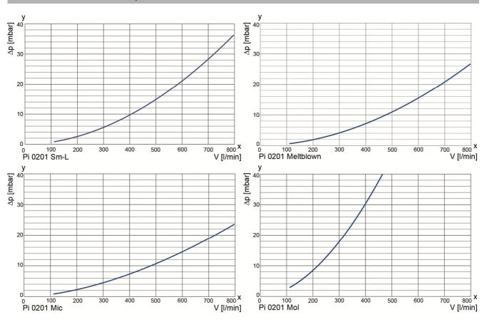
$\begin{array}{l} y = differential \ pressure \ \Delta p \ [mbar] \\ x = flow \ rate \ V \ [l/min] \end{array}$
