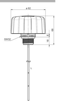
\*1 = version G ¾ with dipstick \*2 = version G ¾ with view inlet and outlet valve, Mol-element L = length of dipstick optional
