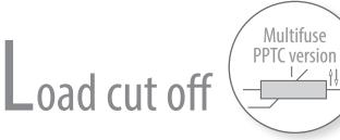
A multifuse (PPTC) works in a similar way like a PTC, which helps to overcome the challenges when switching high loads.
