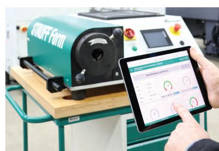
Tube forming machines type SFO-F-A-A can be equipped at the factory with a built-in module for direct connection to a cloud operated by STAUFF. This solution is realised with an integrated SIM card which can be used in all industrial regions of the world.
