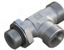
Male threaded studs were designed for female threaded ports in components made of steel. For applications with components made of softer mating materials (e.g. Aluminum), the use of connectors with additionally rolled male threads is recommended.
