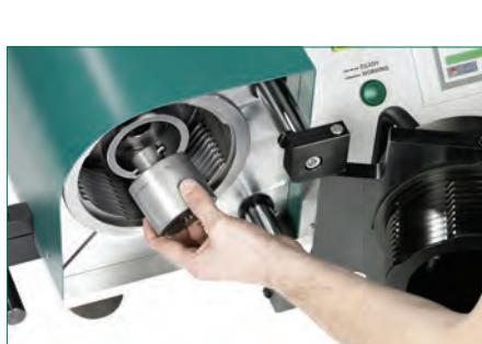
Inserting the tube shaper into the tool holder – with no tools required
