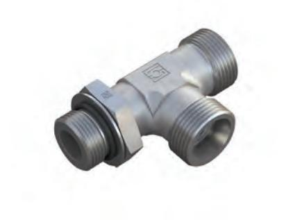
Male threaded studs were designed for female threaded ports in components made of steel. For applications with components made of softer mating materials (e.g. Aluminum), the use of connectors with additionally rolled male threads is recommended.
