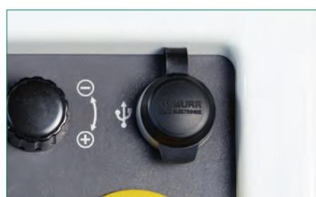
USB connection for maintenance and data input by the manufacturer
