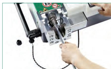
Tooling head for cutting ring assembly based on pre-defined settings / automatic tool size detection
