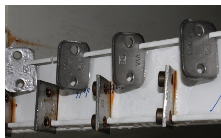
Salt-spray testing of ACT Mounting Hardware (above of the picture) compared to contaminated hardware made of Stainless Steel V4A (below of the picture)
