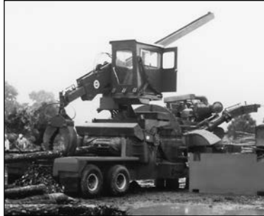
Wichita mechanical PTO handles shock and heavy loads for wood chippers.
