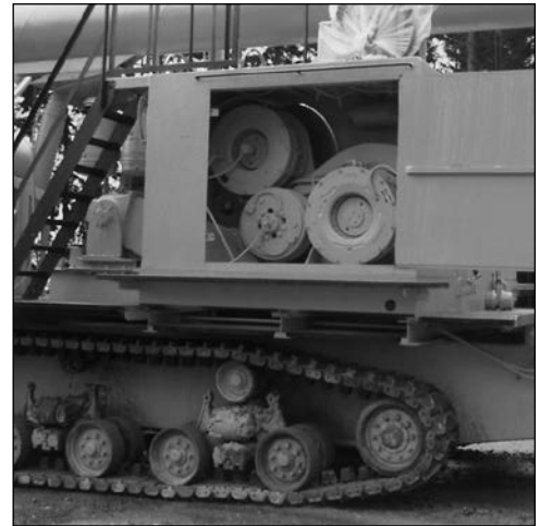
Wichita Kopper Kool Brakes provide precise tension control on winch drives for mobile equipment.
