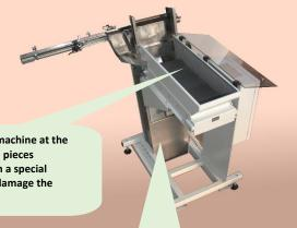
All the parts of machine at the contact with the pieces are covered with a special coating for not damage the pieces
