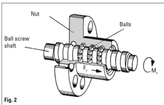
Action: Force  $F_a \rightarrow$  Reaction: Torque  $M_a$
