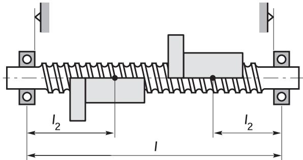
$R_{s2} = \frac{A \cdot E}{l_2 \cdot 10^3} \cdot \frac{l}{l - l_2} \quad [\text{N}/\mu\text{m}] \rightarrow l_2 \leq l/2$ $R_{s2 \min} \text{ at } l_2 = l/2$ |
