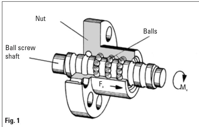
Action: Torque  $M_e \rightarrow$  Reaction: Force  $F_a$
