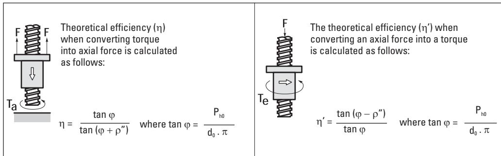
The theoretical level of efficiency is reduced by around 5% to make allowances for operating influences such as speed, temperature and lubrication. If the ratio of load  $F$  to dynamic rated load  $C_{am}$  is less than 0.5, a further reduction is made based on the load factor  $f_l$  (see table below).
