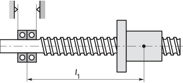
$R_{s1} = \frac{A \cdot E}{l_1 \cdot 10^3} \quad [\text{N}/\mu\text{m}]$ $E = 21 \cdot 10^4 \text{ N/mm}^2$ $I, I_1, I_2 \text{ [mm]}$ |
