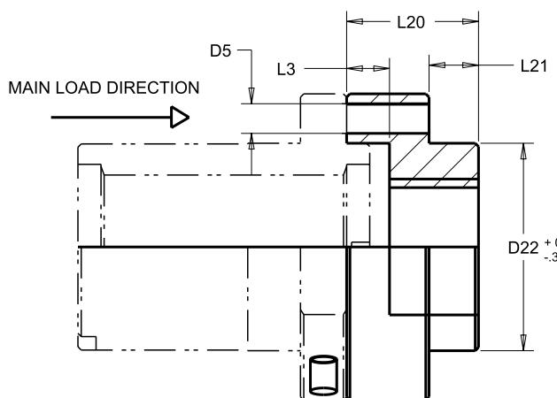
The safety nut is an optional part to a flanged ballscrew. The safety nut basically works just like a normal ballscrew nut. If the axial play increases due to wear, ball breakage or ball loss, the thread of the safety unit comes into contact with the ballscrew. This means the nut cannot be penetrated. The normal function of the unit is guaranteed up to an axial play of 0.5 mm. Thomson also offers complete units with integrated safety nuts. Please ask your Thomson representative.
