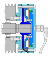
**Stromag KHM** as a shaft-pulley connection. Backlash-free power transmission on pulley side through external body and piston with diaphragm guidance. Friction lining carrier on shaft side with low wearing, wide sliding gear.
