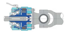
**Stromag KHA** with flexible Periflex<sup>®</sup> VN couplings for drives particularly subject to torsional vibrations. Connection for SAE flywheels. Housings for SAE sizes 1 to 4 possible.
