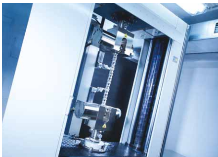
Evaluation of chain breaking strength and elongation up to 1000 kN
