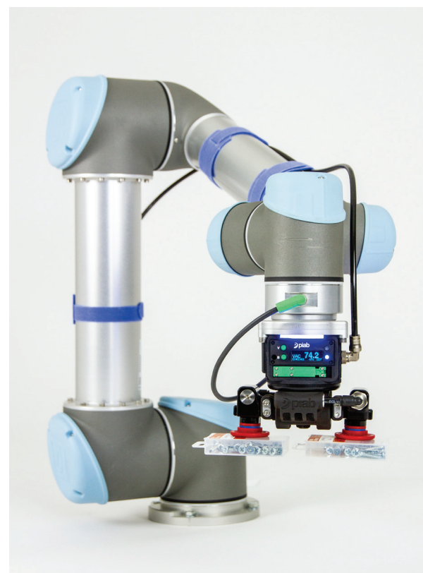
Increased productivity with integrated piSAVE ® Sense valves (object sensing valves), double or single picking of objects.
