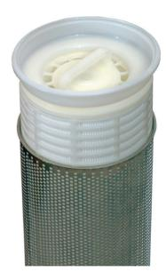
A fully homogeneous welded filter element in one material (Polypropylene or Polyester) with integrated gasket function and length compensation for accurately fitting in the restrainer basket.
