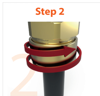
Tighten backnut until a seal is formed onto the cable, then tighten one further turn
