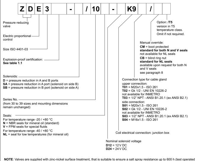
**NOTE**: Valves are supplied with zinc-nickel surface treatment, that is suitable to ensure a salt spray resistance up to 600 h (test operated according to UNI EN ISO 9227 standards and test evaluation operated according to UNI EN ISO 10289 standards).
