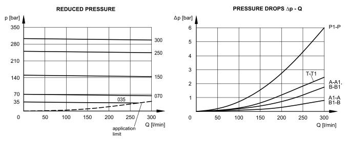
Reduced pressure in P obtained for each adjustment range, with inlet pressure 350 bar and inlet flow 350 l/min.
