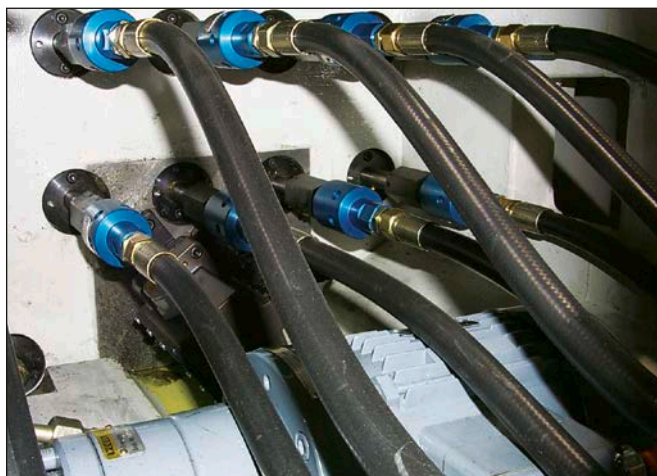
Deublin 1116 Bearing-Supported Unions on Automotive Transfer Line.
