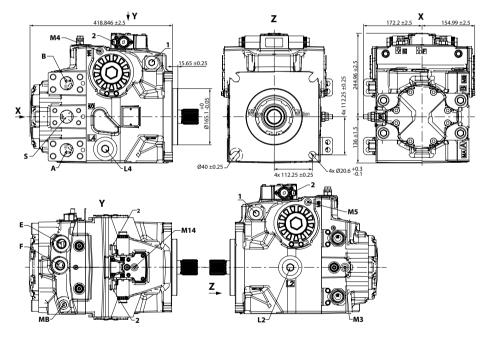
**A/B** system ports: Ø38 mm, 450 bar split flange boss per ISO 6162, M16 x 2; 27 min. full thread depth
