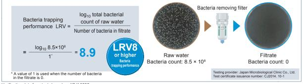
Verification data from tests based on JIS K 3835
