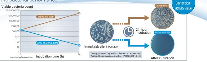
Verification data from tests based on JIS L 1902:2015
