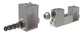
he directional valve RPE2X3-06\*S6 is equipped with inductive position sensors of the working spool. Such valves are used in hazardous equipment where feedback is necessary to ensure safe operation. The sensor is intrinsically safe (protection "i" according to ČSN EN 60079-25). Safe power supply for the sensor and signal transmission must be provided by an appropriate isolating element.
