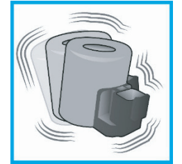
Vibration Test random vibrations according to EN 60068-2-6
