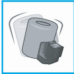
Bumb Test according to EN 60068-2-29
