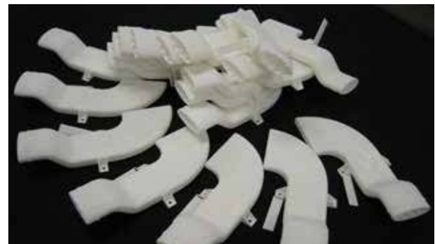
Aircraft air ducting geometry is no longer limited by the means of production so it can be printed lighter and stronger
