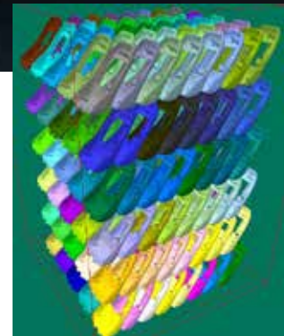
With nesting, hundreds of parts can be printed in a single build, and each one can be unique
