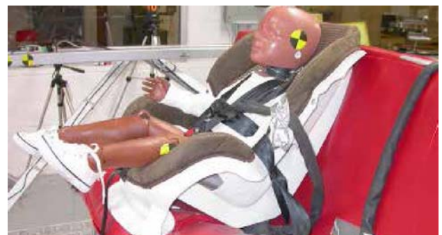
Some 3D printed prototypes so closely match the mechanical properties of production parts that they can be used for crash testing and other functional testing
