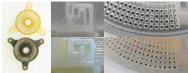
Compare razor sharp edges and corners definition, round circles, minimum feature size, sidewall quality and surface smoothness
