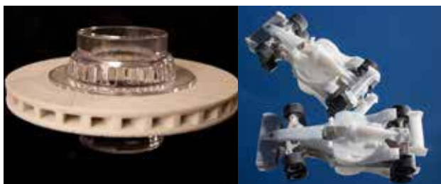
Multi-material composite parts, built in one part/one time
